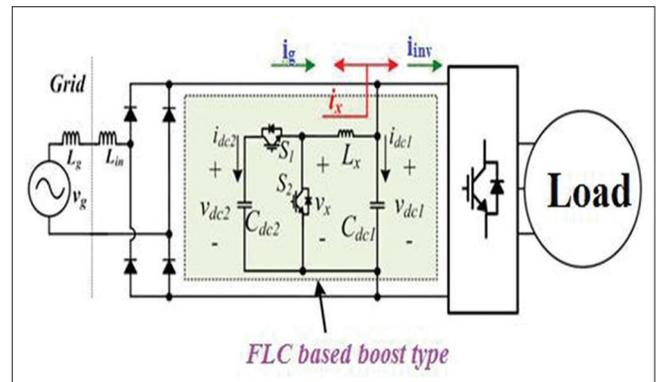
**Figure 2:** Configuration of fuzzy logic controller-based dc-link shunt compensator system.
