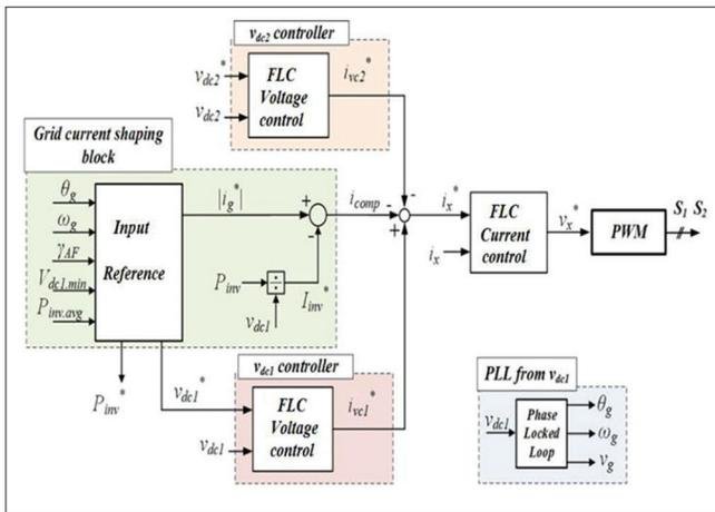
Figure 6: Block diagram of the control method for a single-phase dc-link shunt compensator system
