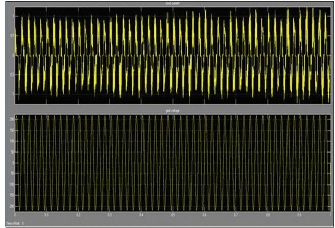
Figure 8: Grid current not in shape for the existing system
