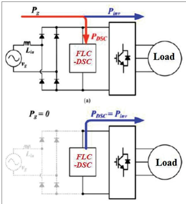
**Figure 4:** Power flow on the conditions of (a)  $T_{GC}$  ( $v_g > V_{dc1.min}$ ) and (b)  $T_{GD}$  ( $v_g \leq V_{dc1.min}$ )
