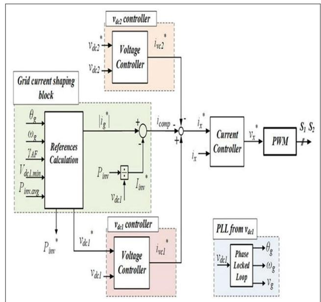
**Figure 5:** Block diagram of the control method for a single-phase dc-link shunt compensator system
