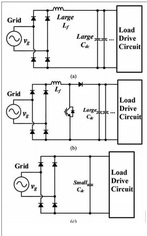
**Figure 1:** Single-phase grid-tied systems with (a) series compensation by filter inductor, (b) cascaded boost converter, and (c) only small dc-link capacitor
