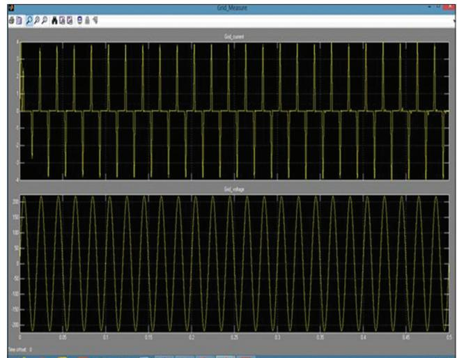
Figure 9: Grid current and grid voltage for interconnecting dc-link shunt compensator
