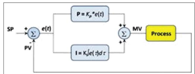
**Figure 3:** Basic diagram of PI controller
