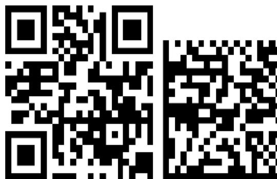
Fig 3: "Pervasive Computing 2007" with the same module size. The left image is using QR Code; the right is using Data Matrix.
